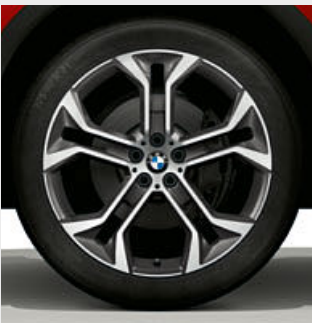
□ 21" light alloy wheels Y-spoke style 744 Bicolour Orbit Grey with mixed tyres and runflat tyres*, gloss-lathed, front 9.5J x 21 with 275/40 R21 tyres, rear 10.5J x 21 with 315/35 R21 tyres.
