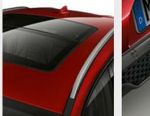
□ The Roof rails in Aluminium satinated provide the base for a multifunctional BMW roof rack unit.
