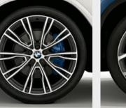
□ 21" BMW Individual light alloy Double-spoke style 718 M in wheels V-spoke style 726 I in Bicolor Cerium Grey matt, bright Bicolor Orbit Grey, bright turned, turned, with mixed tyres and with mixed tyres and run-flat run-flat properties, front 8.5J x 21 properties, front 8.5J x 21 with 245/40 R21 tyres, rear 9.5J x 21 9.5J x 21 with 275/35 R21 tyres.6 with 275/35 R21 tyres.
