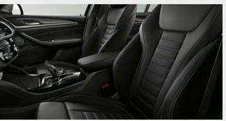
□ The individually adjustable Sport seats for the driver and front passenger feature numerous manual adjustment options, including backrest width, fore-and-aft position, and the backrest and seat angle. Thanks to taller seat and backrest bolsters, and well-defined side bolsters, they provide excellent ergonomics and a high degree of lateral support.
