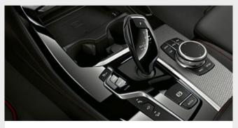
The 8-speed Steptronic Sport transmission offers incredibly sporty gear changes. Whether automatic or manual using gearshift paddles or gear lever – for comfortable coasting or incredibly dynamic driving. In SPORT mode and with the gear lever in the left-hand S/M position, the gear shifts are configured for maximum performance.
