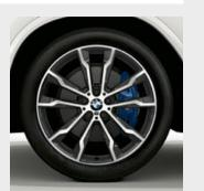
□ 20" M light alloy wheels Double-spoke style 699 M in Bicolor Orbit Grey, bright turned, with mixed tyres, front 8J x 20 with 245/45 R20 tyres, rear 9.5J x 20 with 275/40 R20 tyres.1,2
