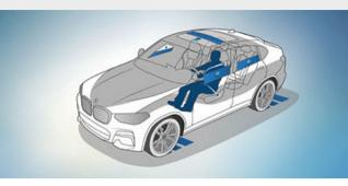
□ Active Protection is a preventive occupant protection system that pretensions the seat belts in critical situations, puts electric seats in an upright position and closes windows and the sunroof, if featured.
