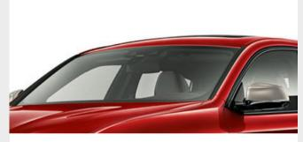
The slight tinted heat/sun protection glazing reflects infrared radiation to prevent the interior from heating up.
