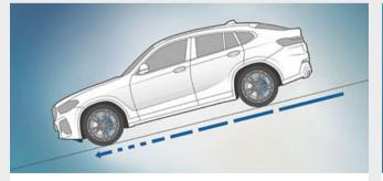
■ The optional **Hill Descent Control (HDC)** in the xDrive models is a system which, when activated, ensures that the vehicle can master the steepest downhill runs automatically and safely at just above walking pace, without the driver having to brake.
