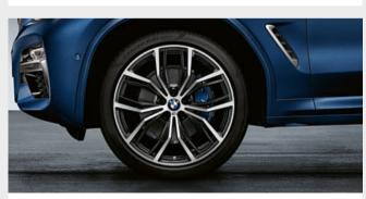
O The high-quality 21" M Performance forged wheels Y-spoke style 701 M are forged, Bicolor matt Jet Black, bright turned, weight-optimised and feature the M logo. Summer complete wheel set with run-flat mixed tyres, wheel size 8.5J x 21 with tyre size 245/40 R21 100Y XL RSC at the front and 9.5J x 21 with tyre size 275/35 R21 103Y XL RSC at the rear.
