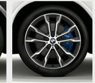
□ 20" M light alloy wheels Double-spoke style 699 M in Bicolor Orbit Grey, bright turned, with mixed tyres, front 8J x 20 with 245/45 R20 tyres, rear 9.5J x 20 with 275/40 R20 tyres.
