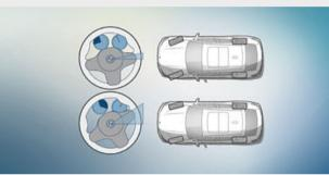
■ The **Variable sport steering** with Servotronic creates a direct and agile steering response and ensures that less physical effort is required to turn the wheel. It reacts to the angle of the steering wheel with varying steering ratios. This improves handling when driving more dynamically and reduces the effort needed to steer when parking and turning.
