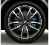
■ 19" M light alloy wheels Double-spoke style 698 M Ferric Grey, wheel size 7.5J x 19 with 245/50 R19 tyres.
