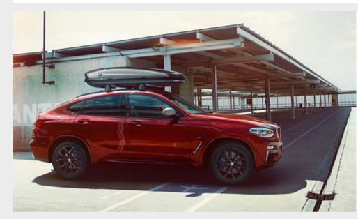
O This contemporary roof box in Black with titanium silver side trims has a 420-litre capacity and fits all BMW roof rack systems. It can be opened from both sides and features triple central locking on each side which makes it easy to load and provides anti-theft locking.
