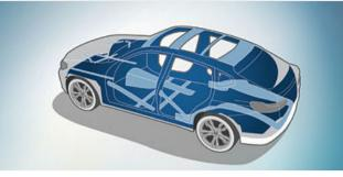
■ The functional structure of the **passenger cell** is composed of a specialised system of beams and nodal connections, featuring strategically deployed high-strength materials so as to deliver maximum passive safety in the event of front, side and rear collisions.
