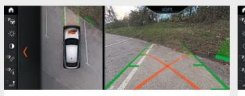
■ The equipment package Parking Assistant Plus<sup>4,\*</sup> makes parking and manoeuvring the vehicle easier. It features Surround View including Top View, Remote 3D View\*, PDC as well as a lateral parking aid, the Active Park Distance Control (PDC), emergency braking function and the Parking Assistant with linear guidance that provides fully automatic parking both parallel and perpendicular to the road.
