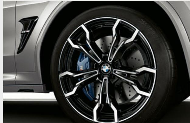
■ Thanks to the use of various materials, M Compound brakes achieve outstanding deceleration values and are extremely stable and highly durable. They also weigh less, which has a positive impact on agility, dynamics and acceleration. The Blue metallic brake callipers with the M designation are the hallmark of these high-performance M specific brakes.
