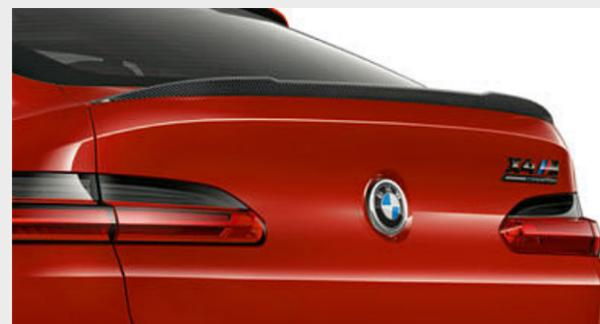
□ The M specific carbon-fibre rear spoiler provides more contact pressure on the rear axle at higher speeds. At the same time, it lends the rear view characteristic sportiness and promises highly dynamic driving experiences.<sup>3</sup>
