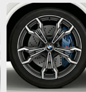
□ 21" M light alloy wheels V-spoke style 765 M Bicolour Orbit Grey with mixed tyres, gloss-lathed, front 9.5J x 21 with 255/40 R21 tyres, rear 10J x 21 with 265/40 R21 tyres.
