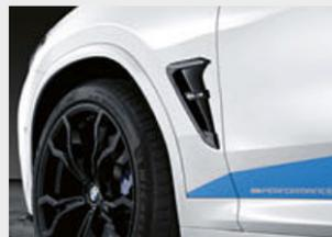
○ Visual highlight on the side of the vehicle: The M Performance Air Breather is made of premium carbon fibre.
