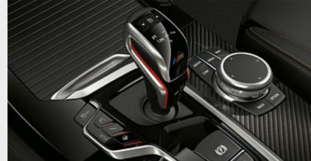
■ The M gear selector switch features a M specific switch pattern. In manual "S" mode, the driver can shift gears manually using the selector lever or the rocker switch on the steering wheel in typical M fashion; in "D" mode, shifting occurs automatically. Whereas the Drivelogic switch for the three shifting programs is on the upper side, the P button for the parking lock is placed under the M logo.
