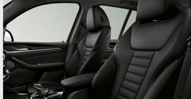
■ The individually adjustable Sport seats with an embossed M logo for the driver and front passenger feature numerous adjustment options, including backrest width, fore-and-aft position, and the backrest and seat angle. Thanks to taller seat and backrest bolsters, and well-defined side bolsters, they provide excellent ergonomics and a high degree of lateral support.
