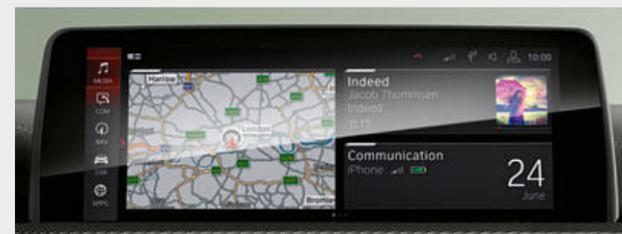
■ The BMW Live Cockpit Professional\* with navigation function includes two high-quality displays consisting of a high-resolution 10.25" Control Display that can be operated by touch and a fully digital 12.3" instrument display. The BMW Operating System 7.0 can also be operated via the iDrive Touch Controller.
