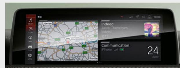
■ The BMW Live Cockpit Professional\* with navigation function includes two high-quality displays consisting of a high-resolution 10.25" Control Display that can be operated by touch and a fully digital 12.3" instrument display. The BMW Operating System 7.0 can also be operated via the iDrive Touch Controller.
