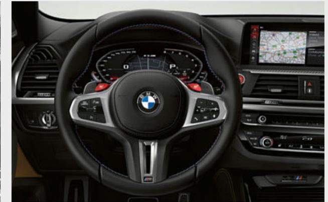
■ The M leather steering wheel including multifunction buttons, the M badge, chrome detailing and an integrated driver-side airbag has the Double-spoke design. Featuring a steering wheel rim in black leather with colour contrast stitching and contoured thumb rests, it feels great in the hand. The driver can also use the M Drive buttons to select the desired settings whilst driving.
