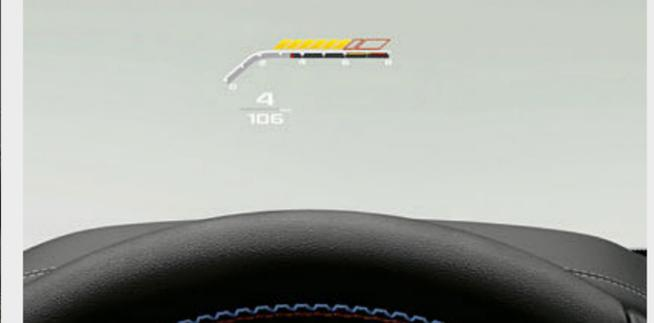
□ The full-colour BMW Head-Up Display<sup>1</sup> incl. M specific display projects information relevant to the journey directly into the driver's field of vision, thereby allowing them to fully concentrate on driving. Information such as the current speed and, depending on the equipment, navigation directions, Speed Limit Info including no-overtaking indicator, along with telephone and entertainment lists are displayed.
