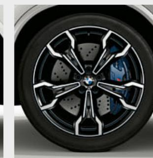
■ 21" M light alloy wheels V-spoke style 765 M in Bicolour Black with mixed tyres, gloss-lathed, front wheel size 9.5J x 21, 255/40 R21 tyres, rear wheel size 10J x 21, 265/40 ZR21 tyres.<sup>1</sup>
