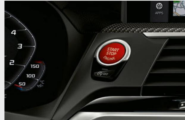
■ The red Start/Stop button allows the engine to be started without using the key once the vehicle has been unlocked. It can also be used to stop the engine. The vehicle key is recognised automatically, without having to insert it.
