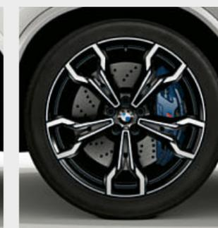
■ 21" M light alloy wheels V-spoke style 765 M in Bicolour Black with mixed tyres, gloss-lathed, front wheel size 9.5J x 21, 255/40 ZR21 tyres, rear wheel size 10J x 21, 265/40 ZR21 tyres.<sup>1</sup>
