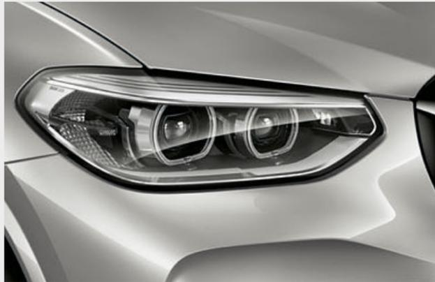
□ The Adaptive LED headlights include low-beam and high-beam headlights and turn indicators with full LED technology. The equipment also features BMW Selective Beam, cornering lights, daytime running lights and Adaptive headlights with variable light control for excellent illumination of the road ahead and better visibility in the dark.
