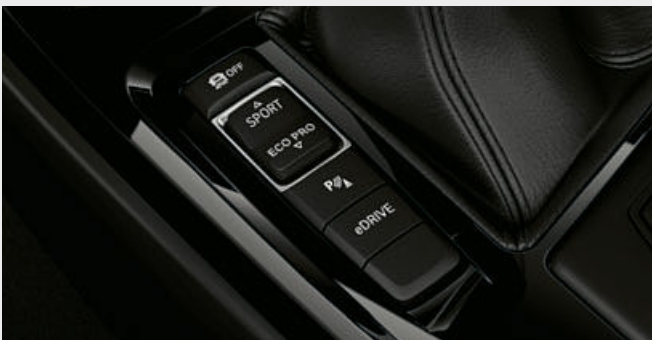
With the driving mode button in the centre console, the AUTO eDrive, MAX eDrive and SAVE BATTERY driving modes can be selected intuitively. At the touch of a button, the driver can quickly adjust the plug-in hybrid drive to different driving situations.
