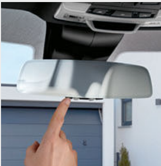
○ This innovative vehicle interior mirror incorporates an adaptive universal remote control for up to three garage doors and property gates.
