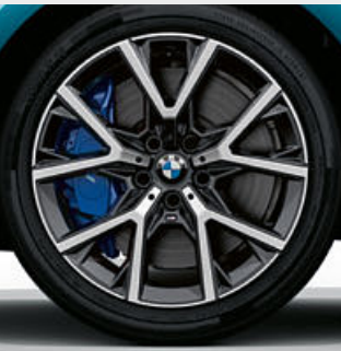
□ 18" M light alloy wheels Y-spoke style 553 M Bicolour Orbit Grey metallic, gloss-lathed, wheel size 8J x 18 with 225/40 R18 tyres.
